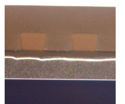
Cross-section of an optical waveguide
